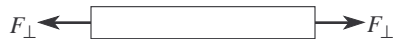
Figure 1 Forces are applied perpendicular to the two ends of a rod: the net force on the rod is zero because the applied forces have equal magnitudes, but opposite directions.
