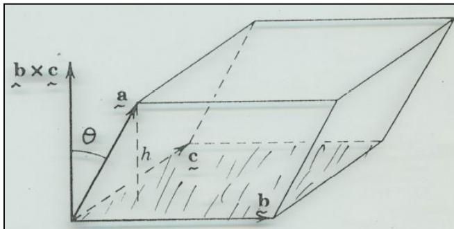
i.e.  $\hat{a} \cdot (\hat{b} \times \hat{c}) = \pm \text{volume of the parallelepiped}$
