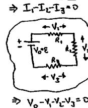
a more complex example, resulting in a larger system of equations, is analysis of a "Wheatstone Bridge" ... (don't worry about detail)
